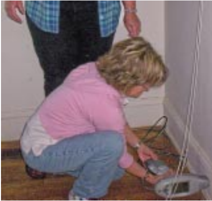
Using XRF to detect lead in paint
